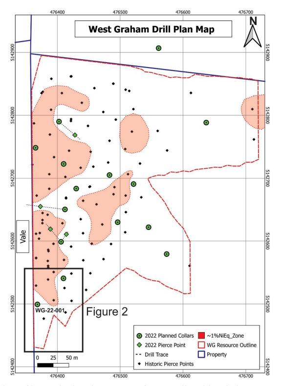
**Figure 1**: Plan map of the West Graham deposit showing pierce points of WG-22-001 and historic holes used in the 2009 resource estimate. Red dashed line is the outline of the West Graham resource projected to surface. Shaded red area are the high-grade zones with NiEq. values of ~1.0%.
