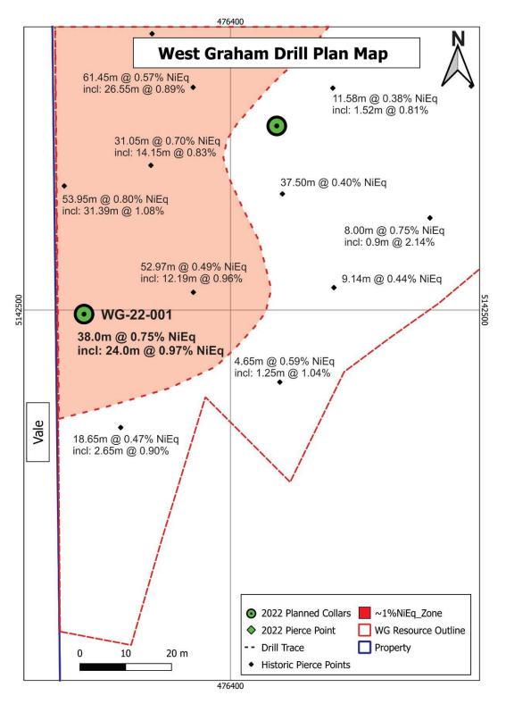
**Figure 2**: Plan map of the West Graham deposit, refer to Figure 1 for the location of the map. Assay intervals include the intersections as reported in the 2009 resource report as well as any high-grade intervals.
